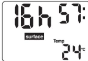
At a depth of 1.2 m/4 ft or less, the display shows “---”. Upon completion of a dive, this is displayed for 5 minutes after which the Digital 330m switches into surface mode. In this mode, the Digital 330m shows SURFACE and the surface interval on the screen. The surface interval will be indicated until it has reached 24 hours or until another dive is performed. In surface mode, the Digital 330m indicates air temperature.
