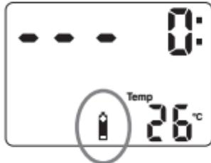
During the start-up phase, the Digital 330m verifies the status of the battery. If the remaining battery charge is 10% or less of the initial charge, the battery symbol will appear on the display for 10 seconds. In this case, the unit must be replaced immediately.
