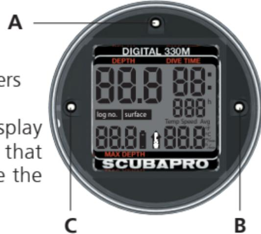
After the 5 seconds in diagnostic mode, the Digital 330m switches into ready mode. After 3 minutes without operation from the ready mode, the Digital 330m turns off to preserve battery energy.
