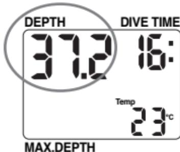
The current depth is displayed in the upper left corner of the screen, in either meters or feet. The depth measurement is calibrated for fresh water according to international standards. Therefore when diving in salt water, the Digital 330m will show a depth slightly greater than actual (2-3% higher). Note that when imperial units are chosen, depths deeper than 999 ft are shown without the leading "1".
