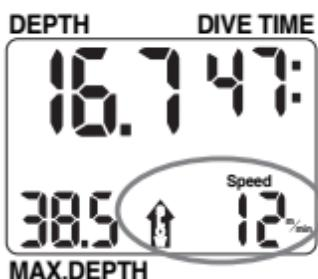
During an ascent, the ascent speed is displayed in the lower right corner instead of the temperature and average depth. The ascent speed is displayed in meters per minute or feet per minute. As soon as the Digital 330m does not detect an ascent anymore, temperature and average depth information appear again. In addition, Digital 330m displays an arrow when it detects a higher than ideal ascent speed. The latter varies with depth as shown in the table.
