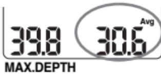
In the lower right corner of the screen, the Digital 330m alternates the display of the water temperature and the average depth. Each value is displayed for 4 seconds at the time. The average depth is continuously updated throughout the dive, and represents the mean value of the depth since the beginning of the dive.
