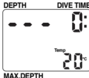
After switching on, all the segments in the display light up for 5 seconds (diagnostic mode): ensure that all segments are lighting up correctly. Do not use the Digital 330m if some segments do not light up.
