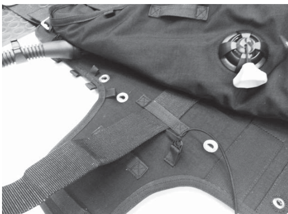
1) Thread the waist belt through the first leash on the back of your harness
