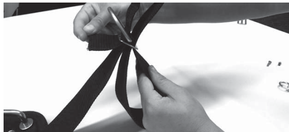
8) Thread the strap back through the first eye of the belt stopper
